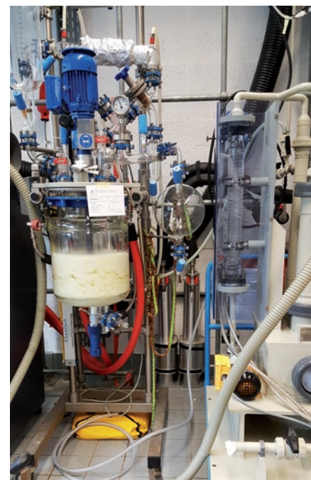
Figure 3: 15 L reactor (left) and gas washer (right)
